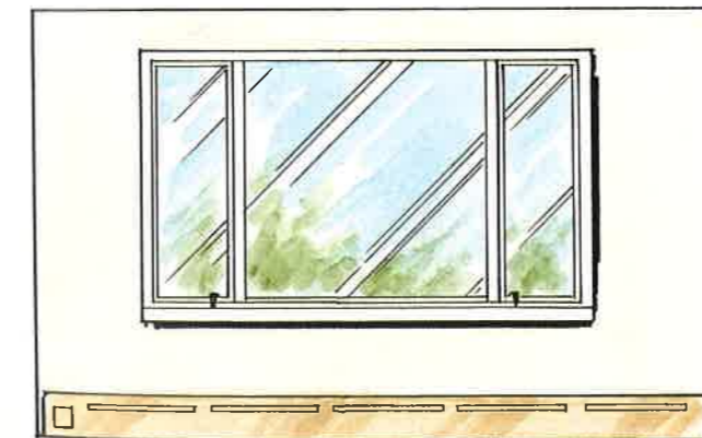
Picture Window with Baseboard Heater
