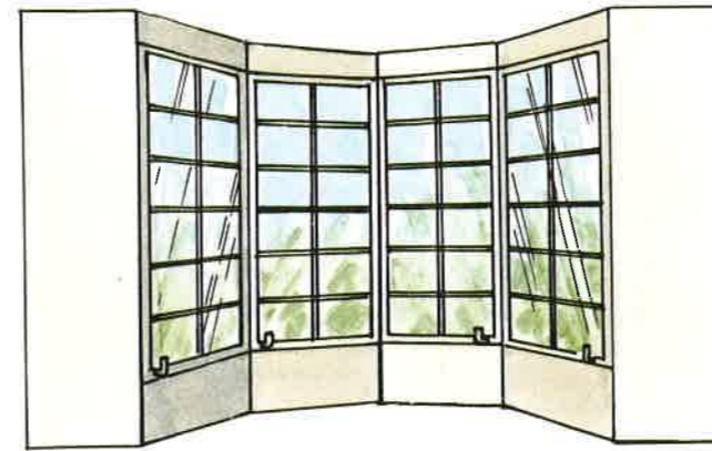
Bay with Casement Windows
